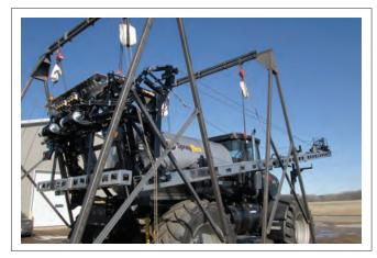
FIG. 63 LIFT BRACKETS (TYPICAL)
