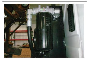
FIG. 96 HYDRAULIC SYSTEM OIL FILTER
