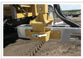
FIG. 87 INNER BOOM PIN BUSHINGS (TYPICAL)
