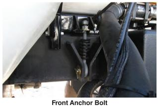
FIG. 65 FRAME ANCHOR BOLTS
