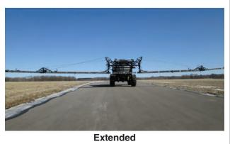
FIG. 51 EXTENDING OUTER WINGS (TYPICAL)
