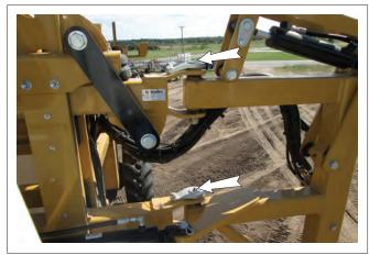
FIG. 86 EXTEND/FOLD PIVOT BUSHINGS (TYPICAL)
