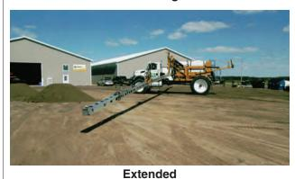
FIG. 46 EXTENDING OUTER WINGS (TYPICAL)
