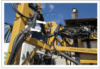
FIG. 85 BOOM TILT PIVOT BUSHINGS (TYPICAL)
