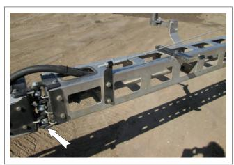
FIG. 89 BOOM BREAK-AWAY BUSHINGS
