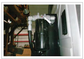
FIG. 92 OIL FILTER INDICATOR
